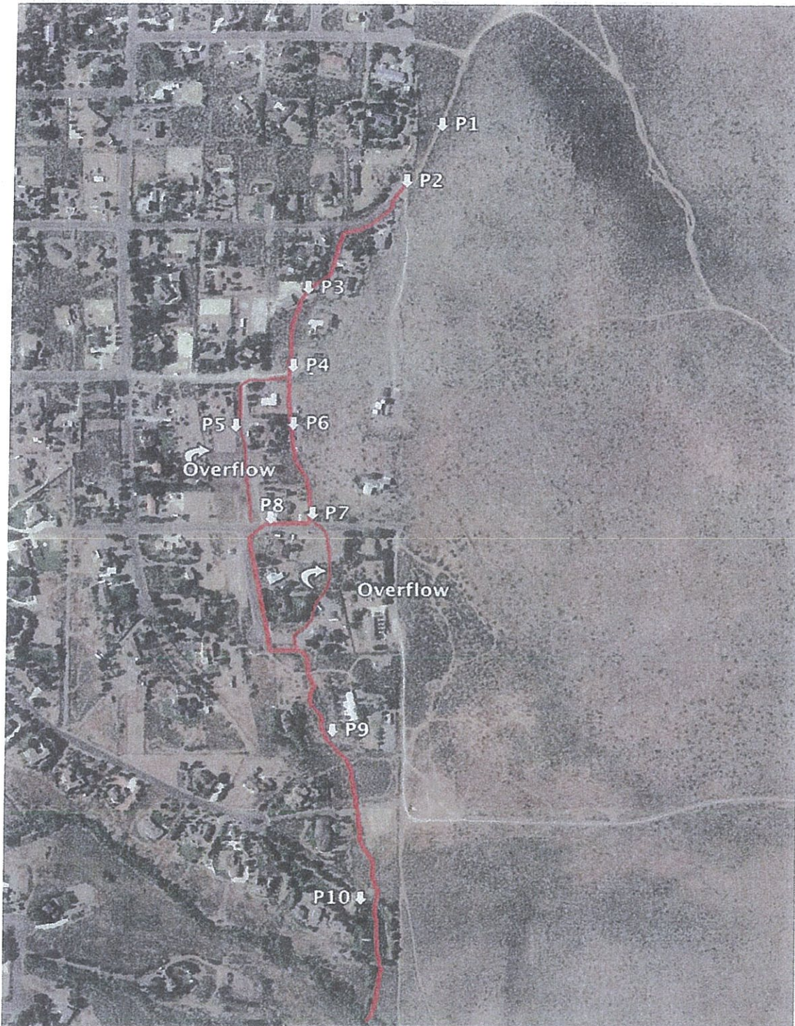
Image3. Goggle Earth image of the flow route that storm water takes from Cedarwood Dr. to Galena Creek. Numbers indicate where photographs are taken.
