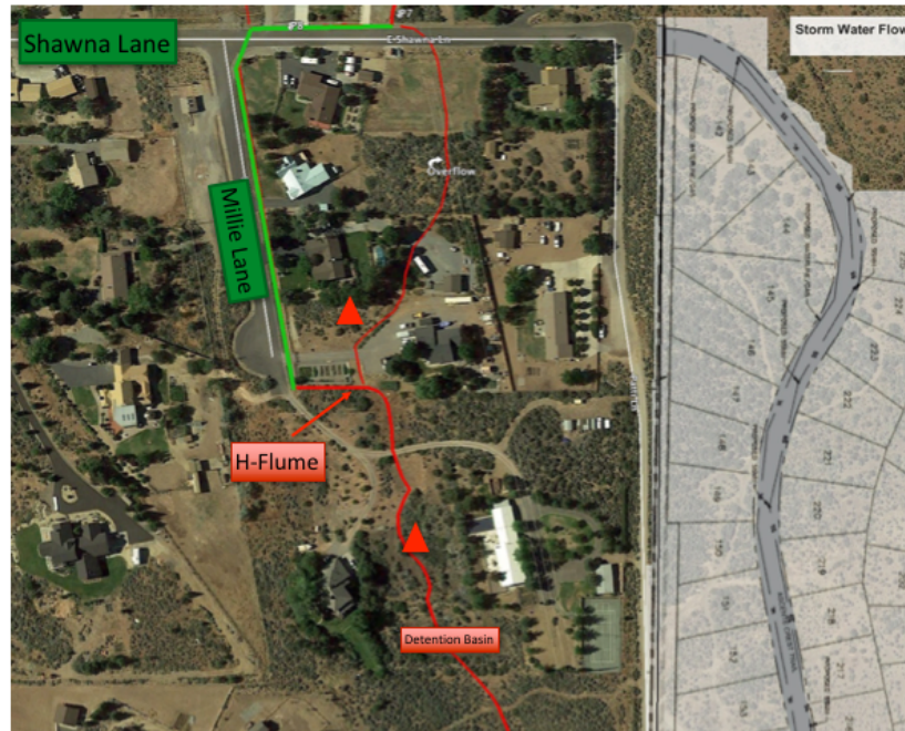
Flow Path of Ascente's storm water, Shawna Lane to Private Detention Basin
